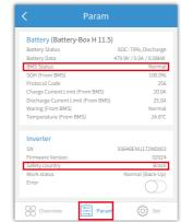
Note: For compatible lithium batteries, BMS status will display "Normal" after selecting the right battery company.
