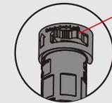
Press the button and hold it to unlock when unplugging AC terminals.
