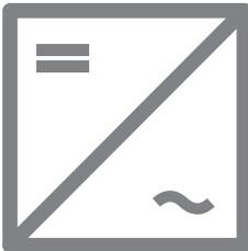
The system contains additional PV inverters that convert the direct current from the PV modules into grid-compliant alternating current. The hybrid inverter can convert the power generated by the PV inverters into direct current and feed it to the battery. In secure power supply and battery-backup operation, power generated by additional PV inverters cannot be used.
