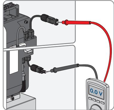
5. If the voltage of a battery module is below 90 V, check and update the firmware version of the Sunny Boy Smart Energy (see Section 2.4.1, page 7) or of the Sunny Tripower Smart Energy (see Section 2.3.1, page 6).
