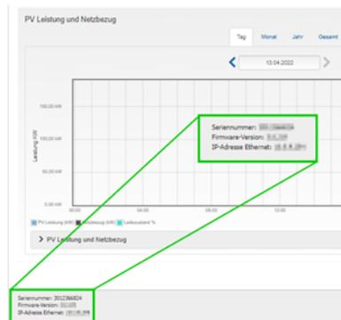
2. If the firmware version is  $\leq 3.04.16.R$ , update the firmware to version  $\geq 3.05.26.R$  (see inverter manual). In the firmware 3.05.26.R for the inverter, the firmware version 1.1.20.R for the battery is also included. This is required for faultless operation.
