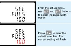
Use M and P buttons to choose pulse rate, then press E L to confirm the setting and press VIL to return to
