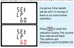
Press and p to select the time interval. Then press to confirm the set-up.
