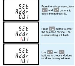
Press E 🕹 to confirm the setting and press 🎶 🚉 to return to
