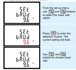
Press E 🕹 to confirm the setting and press 💯 🚉 to return to
