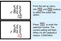
Use M A and P buttons to choose pulse rate, then press  $\fbox{\sc B}$  to confirm the setting and press  $\fbox{\sc U1\_}$  to return to the main set up menu.
